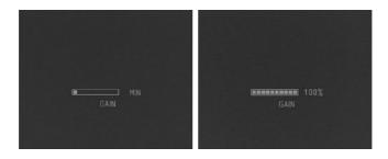
Thermal sensitivity adjustment improves the quality of the observed image depending on the contrast of the observed object and the background temperature the device due to the manual adjustment of the core (micro-bolometer) sensitivity.
