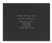
The image is moved by pressing buttons A and B. The axis are switched by pressing shortly button M. The active coordinate is framed. The display shows X and Y coordinates with respect to the screen center. Match the target center with the reticle center.
