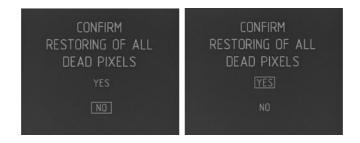
To exit the correction menu select option "Exit" and press and hold (more than 2 sec.) button M.
