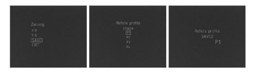
Using buttons A and B select the profile number and press and hold (more than 2 sec.) button M to save the zeroing results, and the display will show the message confirming the profile is saved.
