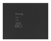
To exit the zeroing menu press and hold (more than 2 sec.) button M on the Exit option.
