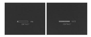
**Thermal sensitivity adjustment**. In the sensitivity menu select the required thermal sensitivity level by pressing button A or B. Press and hold (more than 2 sec) the button A to enter the main menu or exit the adjustable parameters menu by pressing shortly button M.
